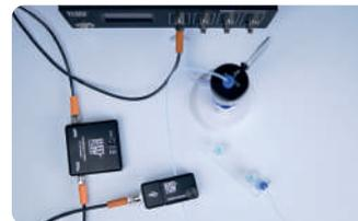
This sensor detects **the presence of fluids inside clear tubing, triggers a signal to another instrument**, and acts as needed - stop, wait, allow enough flow to clear the tubing, or reset the sensor.
