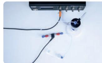
Flow-through pressure sensors adapted to gases or liquids, and compatible with the Luer-lock standard. The flowplus fluid sensor is intended to **measure the pressure** of fluid media flowing through the sensor.
