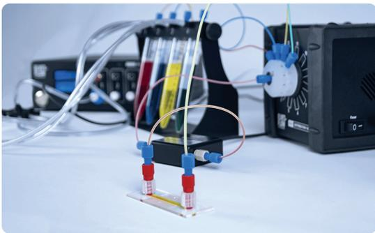
The **Sequential Injection Pack** includes all the necessary elements to sequentially inject up to 12 (or more) solutions in a fully automated fashion using our computer-controlled 12 to 1 MUX Distribution bidirectional valve.
