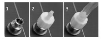
Note that the supplied particle/humidity filter must be placed between the pressure outlet of the AF1 Pressure Generator and the pressure inlet of the AF1 Pressure Controller. The arrow on the filter indicates the direction of airflow: from the Generator to the Controller. Note: the stand is not available for purchase.
