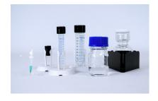
Microfluidic Reservoirs microfluidic adapters for eppendorf ©, falcon © tubes or gl45 threaded glassware
