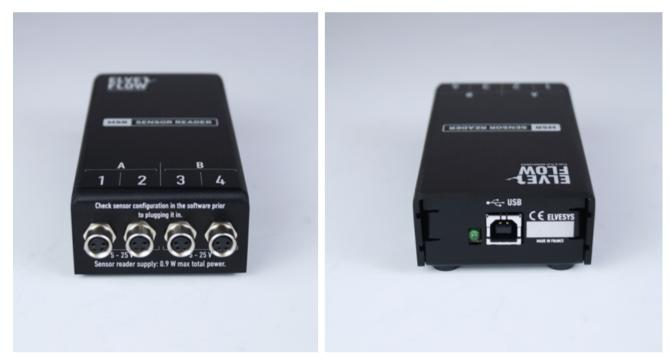
Front side (left) with four 4-pin female connectors to be used with any Elveflow pressure or flow sensor model. Rear side (right) with a USB connector.
