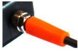
2. Connect the male part of the cable to the female connector on your instrument.
