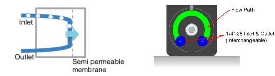
The Elveflow Bubble trap should be connected to the flow path through the ¼-28 receiving ports designed on the round PVC part, using the ¼-28 fittings provided. Inlet and outlet are interchangeable. When a liquid containing bubbles is flown through the Elveflow Bubble trap, the aqueous fluid is retained, while bubbles are automatically expelled through a microporous hydrophobic PTFE membrane, resulting in a bubble free liquid coming out of the device.
