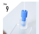
Use the supplied 1/32" OD tubing to connect microfluidic tanks with the chip.
