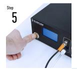
Turn on the OB1 by pressing power switch on the front side of the instrument.
