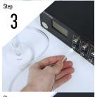
Plug microfluidic tanks to the OB1 pressure controller outlet. The Elveflow reservoirs connection instructions are covered by a specific guide (see Elveflow Microfluidic reservoirs assembly Instructions).
