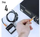
If you bought flow sensors, connect them to OB1 for the feedback loop and between microfluidic tanks and chip for flow measurements.
