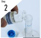
Fill your microfluidic tanks with dispersed (water) and continuous phase (oil).
