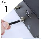
Connect your OB1 pressure controller to external pressure supply using pneumatic tubing and to computer using USB cable
